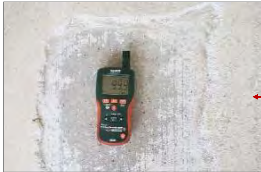
Testing current conditions for concrete in both pools – high levels of moisture recorded
