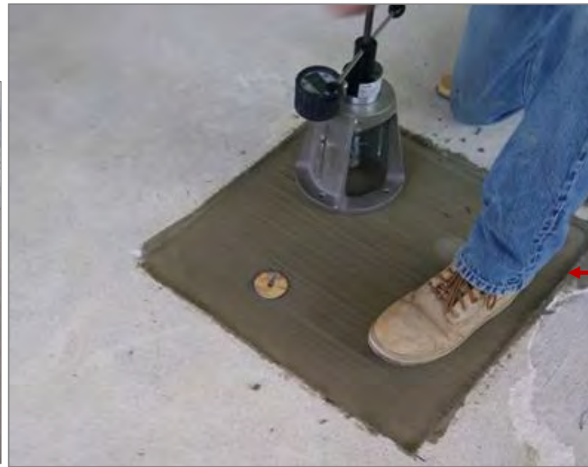
Testing of materials for pool treatment over moist concrete
